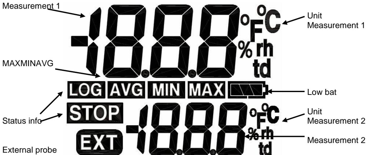
**Measurement 1** displays the current relative humidity(Log110) or the current temperature(Log100).
