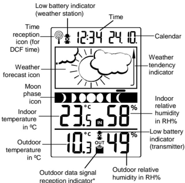
\* When the signal is successfully received by the weather station, the outdoor transmission icon will be switched on. (If not successful, the icon will not be shown on LCD). The user can then easily see whether the last reception was successful (icon on) or not (icon off).
