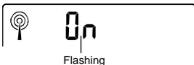
In areas where reception of the DCF time is not possible, the DCF time reception function can be turned OFF. The clock will then work as a normal Quartz clock. (Default setting is ON).
