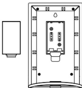
1. Insert finger or other solid object in the space at the bottom center of the battery compartment and lift up to remove the cover.
