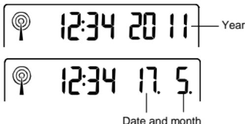
The date default of the weather station is 1. 1. 2011. Once the radio-controlled time signals are received, the date is automatically updated. However, if the signals are not received, the date can also be set manually.
