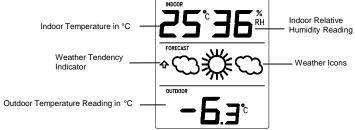
Immediately after inserting the batteries into the receiver, all the segments on the LCD screen will light up briefly, before displaying the indoor and outdoor temperatures and humidity readings as well as the sun with cloud icons.
