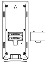
The Weather Station uses 2 x AA, IEC LR6, 1.5V batteries. To install and replace the batteries, please follow the steps below:
