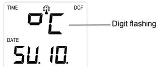
The temperature display can be selected to show temperature data in °C or °F (Default °C).
