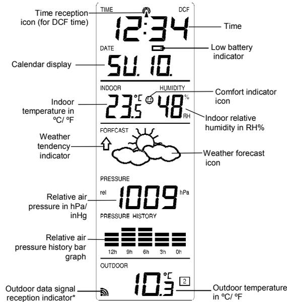
\* When the signal is successfully received by the weather station, the Outdoor reception icon will be switched on. (If not successful, the icon will not be shown in LCD) So the user can easily see whether the last reception was successful (icon on) or not (icon off). On the other hand, the flashing of the icon shows that a reception is being done now.
