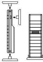
The Transmitter is supplied with a holder that may be attached to a wall with the two screws supplied.
