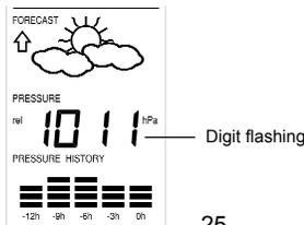
The default relative pressure value is 1013 hPa (29.92 inHg). This can be manually set to another value within the range of 960 – 1040 hPa (28.35 – 30.72 inHg) for a better reference.
