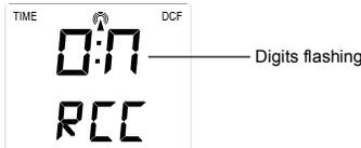
In area where reception of the DCF time is not possible, the DCF time reception function can be turn OFF. The clock will then work as a normal Quartz clock. (Default setting is ON).
