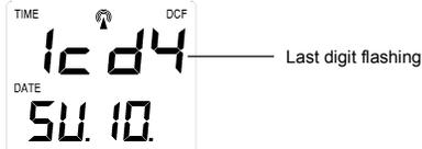
The LCD contrast can be set within 8 levels, from LCD 0 to LCD7 (Default setting is LCD 4):
