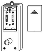
The Thermo-Hygro transmitter uses 2 x AA, IEC LR6, 1.5V batteries. To install and replace the batteries, please follow the steps below:
