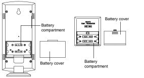
First, insert 2 x AA, IEC LR6, 1.5V batteries into the Weather Station. Once the batteries are in place, all segments of the LCD will light up briefly. Then the indoor temperature, the time as -:--, and the weather icons sun and clouds will be displayed. If the indoor temperature is not displayed after a few seconds, remove the batteries and wait for at least 30 seconds before reinserting them. Once the indoor data is displayed proceed to step 2.
