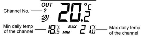
To view the daily MIN and MAX temperature of another channel, user shall press the CH key to shift to various channel display.
