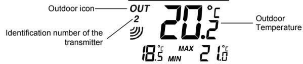
The bottom LCD section shows the outdoor temperature and the transmitter number.
