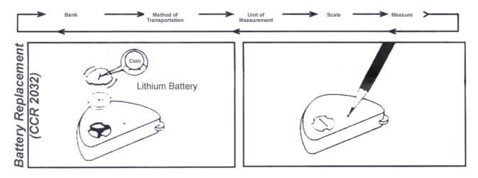
Turn the Map Measure off before replacing the battery. Use a coin to open/close the battery lid.
