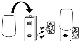
The Thermo Hygro Sensor is supplied with a mounting bracket and two screws for wall mounting. Be sure to differentiate each of the Sensors since they are not numbered and have no specific order for setup (also see **6.1 Basic Setup<sup>2)</sup>**).
