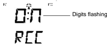
In area where reception of the DCF time is not possible, the DCF time reception function can be turned OFF. The clock will then work as a normal Quartz clock. (Default setting is ON).
