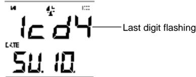
The LCD contrast can be set within 8 levels, from LCD 0 to LCD7 (Default setting is LCD 4):
