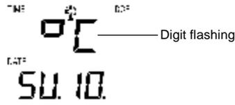
The temperature display can be selected to show temperature data in °C or °F (Default °C).
