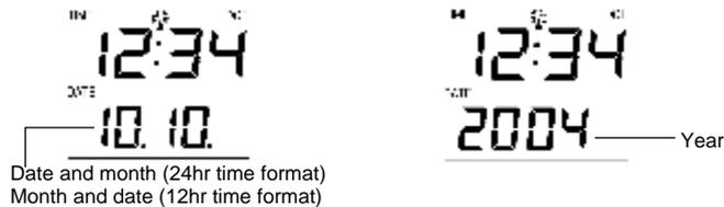
The date default of the Weather station is 1. 1. in the year 2004. Once the radio-controlled time signals are received, the date is automatically updated. However, if the signals are not received, the date can also be set manually.
