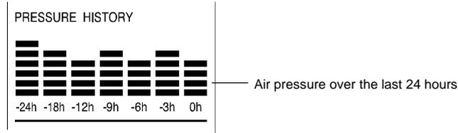
The bar chart indicates the air pressure history trend over the last 24 hours in 7 steps, 0h, -3h, -6h, -9h, -12h, -18h and -24h. The "0h" represents the current full hour air pressure recording. The columns represent the "hPa" (0, ±2, ±4, ±6) at specific time. The "0" in the middle of this scale is equal to the current pressure and each change (±2, ±4, ±6) represents how high or low in "hPa" the past pressure was compared to the current pressure.
